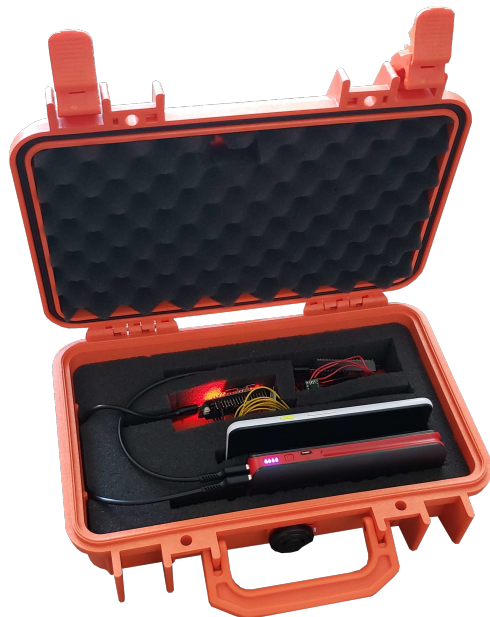
Figure 4.2. The sensor platform containing a BLE-enabled microcontroller, a cellular modem, and a GPS- and LoRa-enabled microcontroller.
