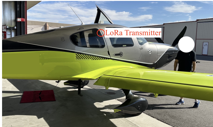
Figure 5.2. Small aircraft broadcast platform. We carried a LoRa transmitter on a Cirrus SR22 and flew it around Las Vegas, Nevada at altitudes from 1.7 km–3.3 km. The climb rate was 6 meters per second.
