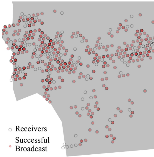
(a) Receiver coverage in San Diego from a single weather balloon deployed in the San Diego area.
