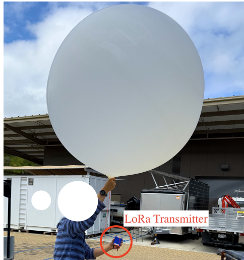
Figure 5.1. Weather balloon broadcast platform. We attached a LoRa transmitter to three weather balloons and flew them up to 15 km above San Diego, California. The climb rate was 0.020 meters per second.
